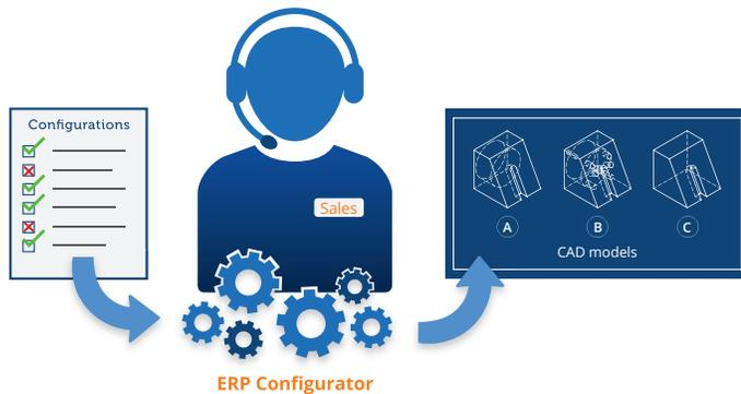
ConfigLink allows the user to push ERP configuration parameters to parametrically configure 3D models and produce 3D images and drawings of configured product.
